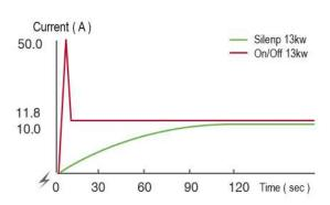
With its smart conversion, Silenp can be applied to a wide range of voltage which is 180-260V.
